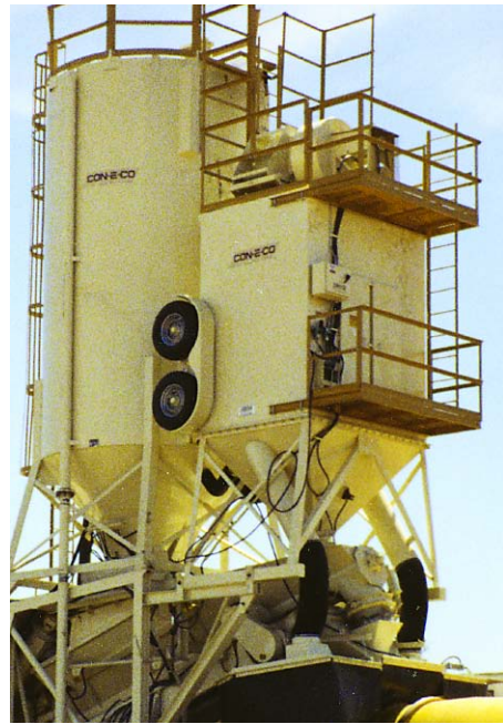
Mobile central dust control
