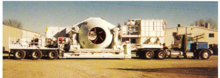
Mobile tow-away self-erecting tilt mixer.
