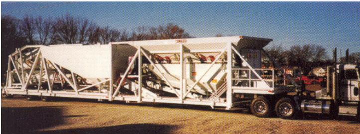
Mobile tow-away self-erecting batch plant.
